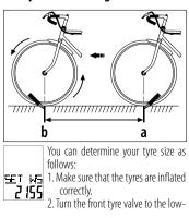
est position and mark the position of the valve on the ground (a). Move the bicycle forward by one tyre rotation, until the valve has reached the lowest position
